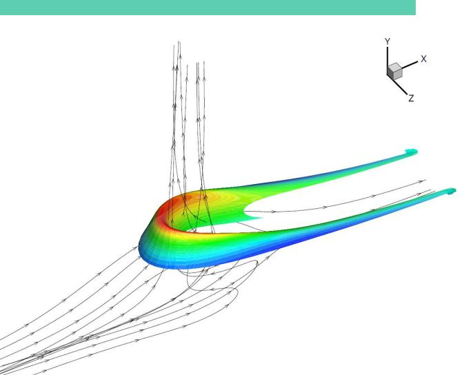
Particles initially located on a horizontal plane close to the wall are advected in time, and the plane is colored with  $\rho_{t_0}^t$ . It is observed that the criterion seems to capture most repelling particles from the wall.
