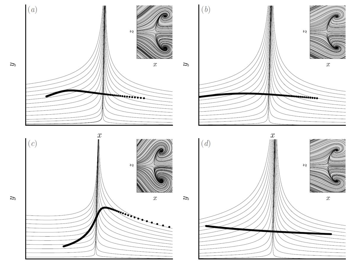
Using the method of Perry & Chong [2] with the procedure developed by Surana [3], we obtain 3D separartion patterns of incompressible flows. The wall shear-stress is given by the skin-friction trajectories:
