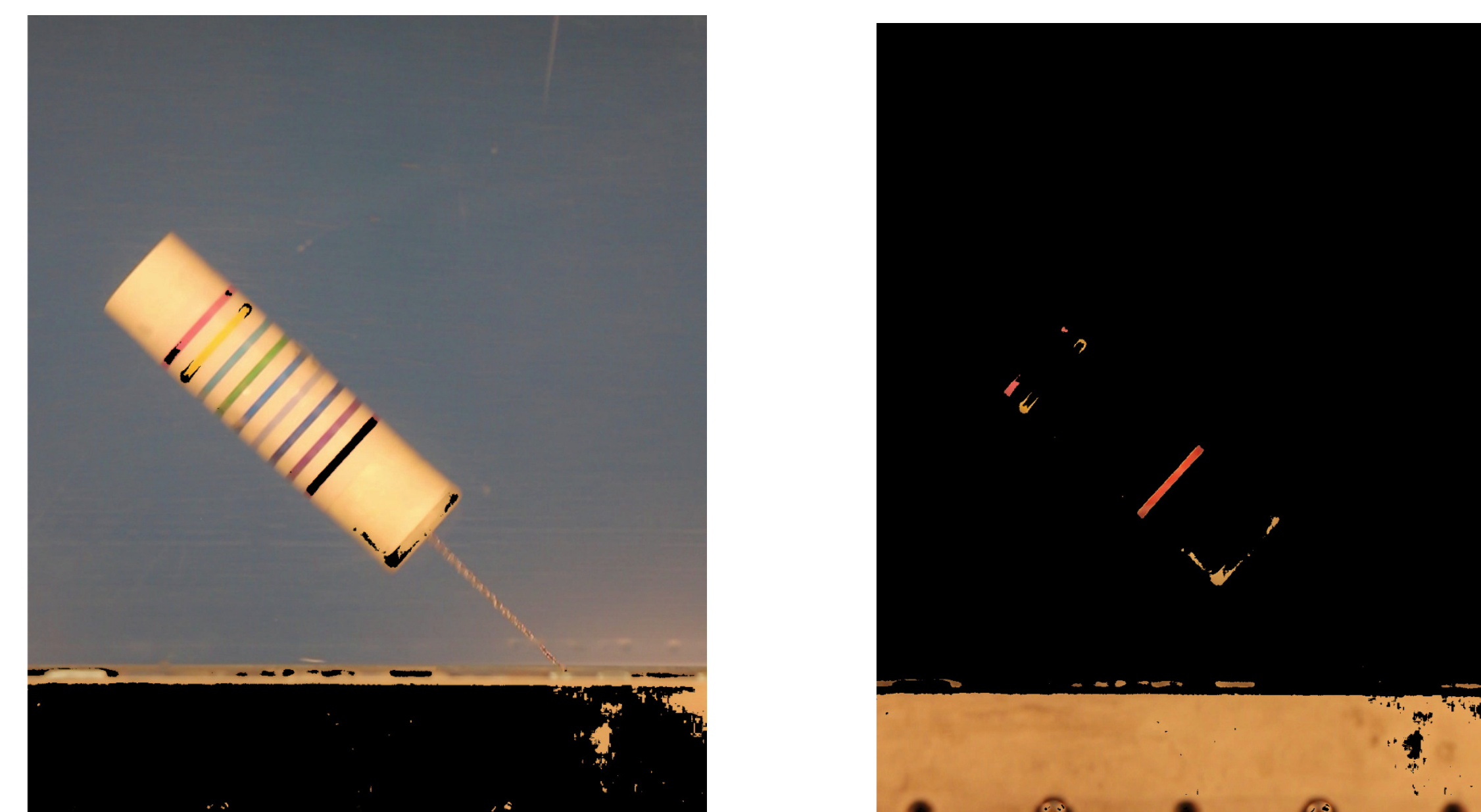
Recognition of a specific color (filtered image and its negative) with OpenCV library
