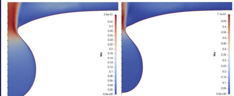
Simulation of an arbitrary volume of fluid changing shape because of surface tension forces (including contact angle)
