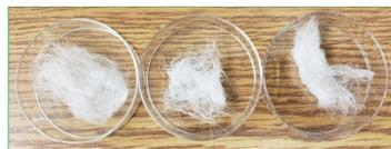
Figure 3. Different samples produced using our CS setup in different conditions. The solution was PVP solved in ethanol.
