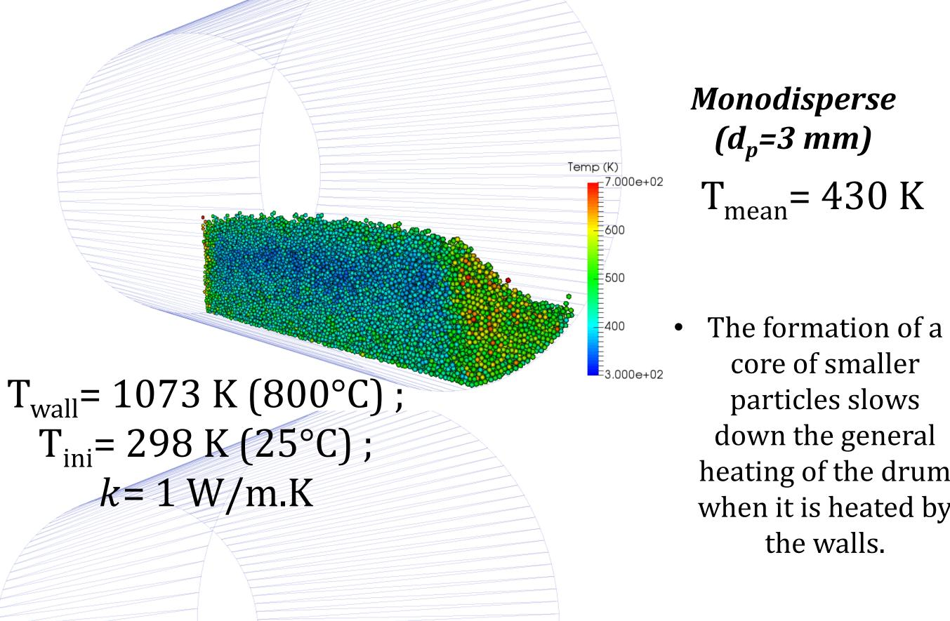
core of smaller particles slows down the general heating of the drum when it is heated by the walls.
