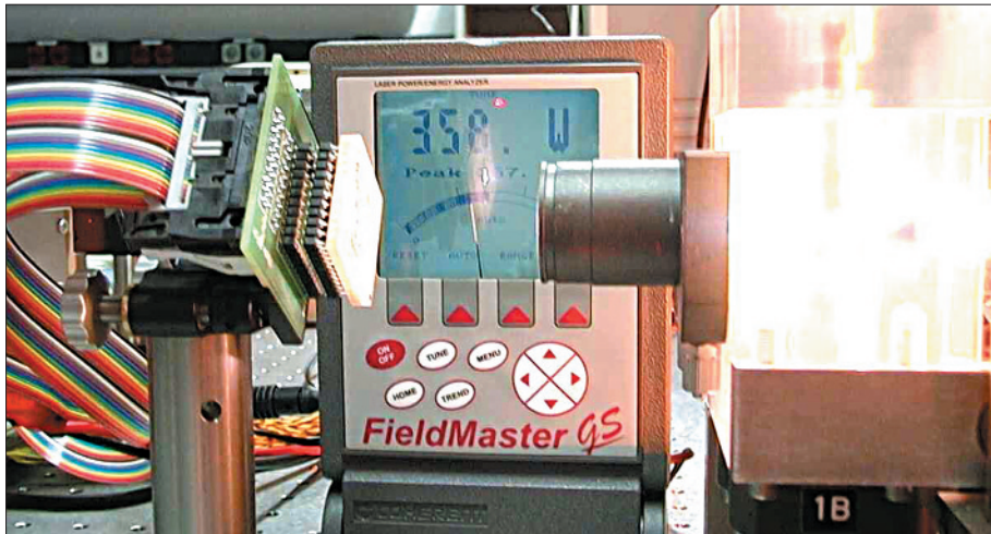
1. Power to the people: the flexible membrane mirror handles up to 500 W of continuous-wave YAG power.
