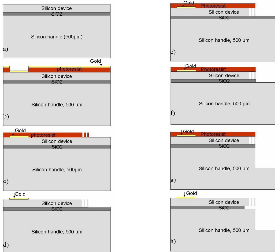
Fig. 9. Process flow for the microfabrication of the tunable vertical silicon grating.
