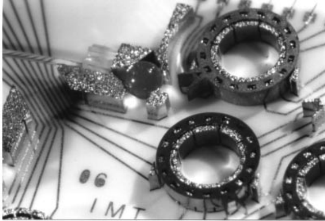
Figure 2.1.27. Close-up view of fully assembled 2 \times 2 switch matrix.
