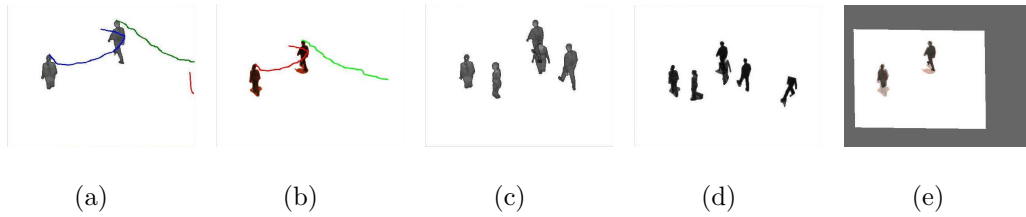
Figure 1: Illustration of processing steps for a given frame. (a) and (b) Object trajectories in IR and visible respectively, (c) and (d) Foreground composite image in IR and visible respectively, (e) Registration result
