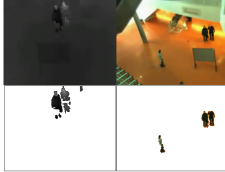
Figure 9: Top: a thermal and a visible video frames (Frame 300, Seq.8), Bottom: corresponding thermal and visible foreground images
