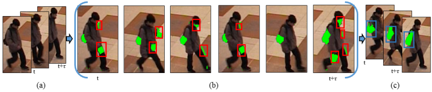
Figure 3: Carried object detection. (a) Input video (frame t to t + \tau ). (b) CO candidate regions (red bounding boxes show the spurious candidates). For clarity only highly probable CO regions are shown in the figures (green segmented regions). (c) Detected COs delineated by blue bounding boxes.
